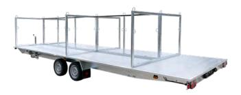
Large transport trailer for 12 portable toilets. The trailer features a lightweight aluminum platform on two axles, which ensures maximum durability and easy maneuverability.
