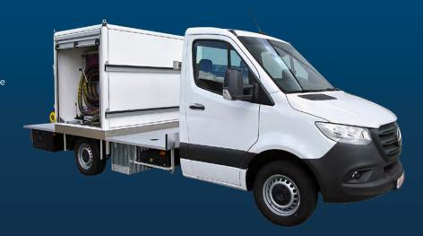
GLOBAL FXD Units are our fixed superstructures for the truck (waste disposal vehicle) of your choice. The pump is driven either by the PTO of the vehicle's hydraulic system or an external motor.
